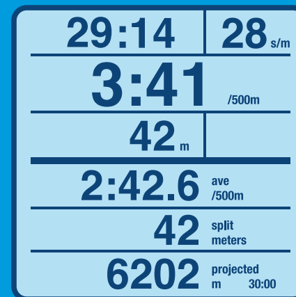
The monitor has been programmed for a timed piece. The bottom read-out is predicting how far the rower will go.
